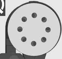
Press carefully the fuzzy side of sanding disc against the packaging pad, as firmly as possible.
