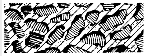
OPEN COAT (1/3 LESS GRAIN THAN CLOSED)
