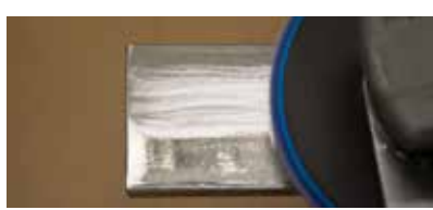
Supersize layer for a cooler cut & reduced heat generation during use, providing better part quality and no burn marks
