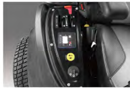
1 Our control panel has integrated fuel management technology, usage hour meter, maintenance reminders and many other features.
