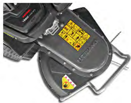
The string trimmer head is offsetted to one side to remove weeds at the root of obstruct easily.
