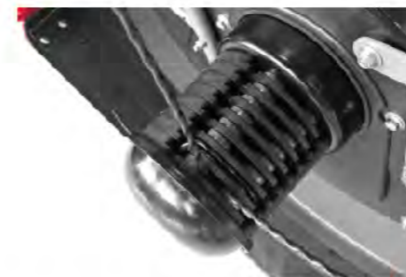
String's position is easy to change from 2"-5.4" on desire to get different stubble heights.
