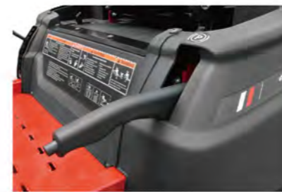
3 A park brake handle equipped for easily one-handed operation
