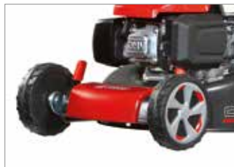
Independent cutting height adjustment on each wheel.
