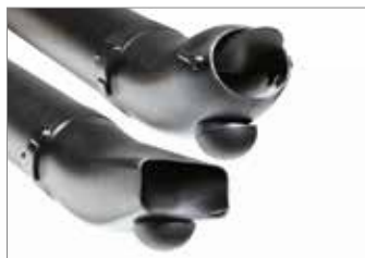
Two air delivery nozzles supplied as standard: rectangular/round section, both equipped with hemispherical support so the tube can rest on the ground on level terrain to reduce operator fatigue (SA 9010).
