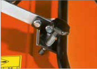
Working depth adjustment spring. Always maintains the preset position.
