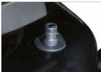
The quick-fit "Deck Wash System" connector on the mowing deck makes it possible to direct water inside the deck for quick and easy cleaning of the cutting mechanism (84).
