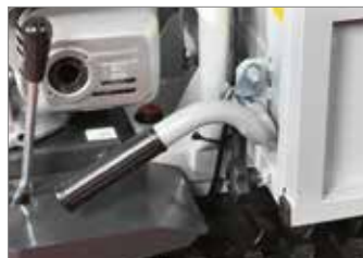
Manual dump with automatic locking system.
