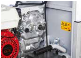
Independent 2100 rpm PTO.
